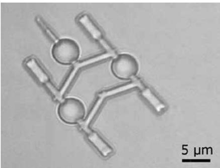
An optical image of an optically trapped probe.
