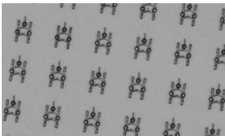
An array of micro-tools on a glass surface before they are transferred into a sample cell.
