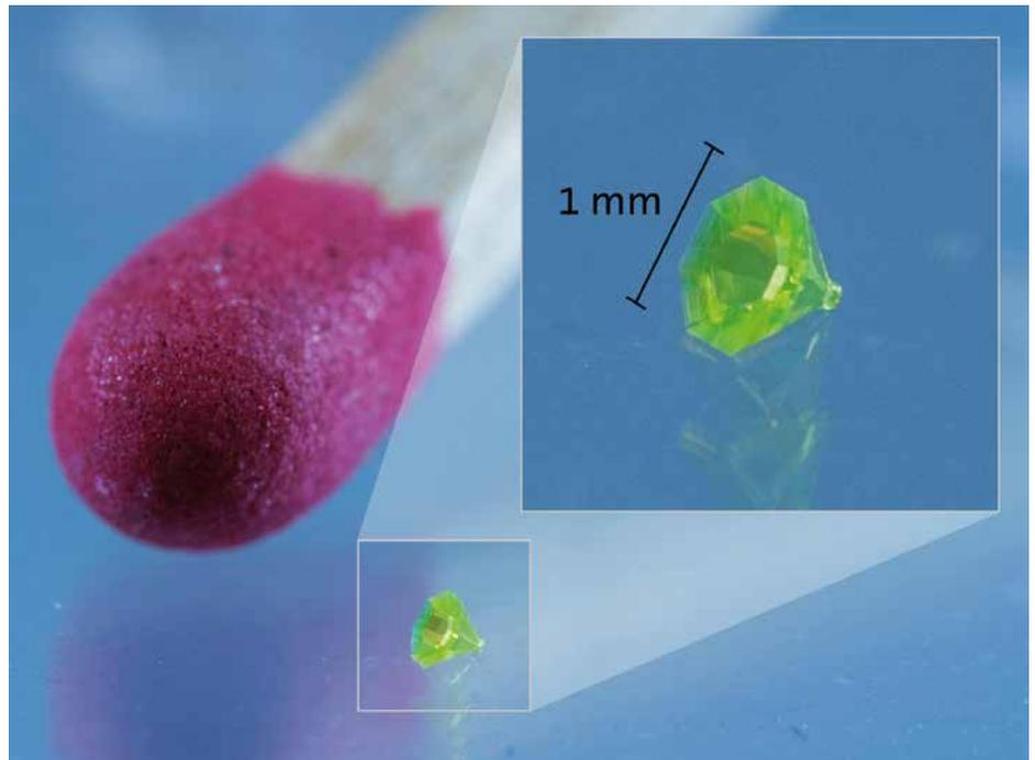
Prototype of a miniature nozzle with a diameter of one millimeter fabricated for the precise formation of liquid micro-droplets.
