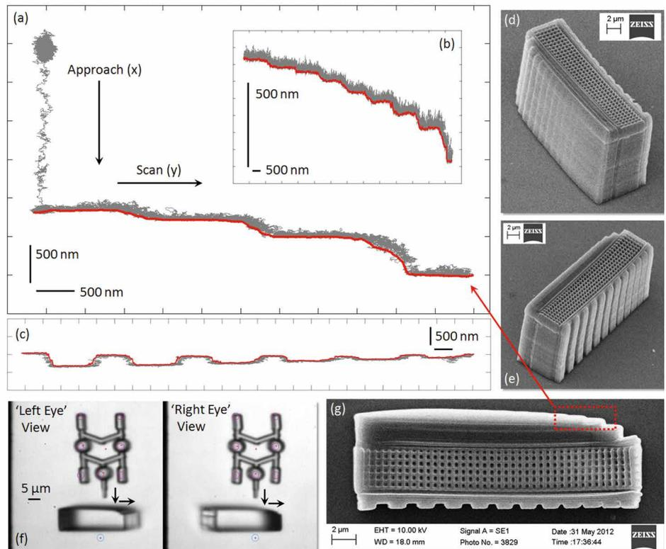
Measurement of the surface topography of a test sample.
